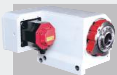
Workhead C-axis (Option) With special software, and C-axis can do the non-circular grinding and thread grinding.
