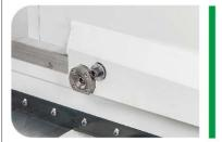
The work head is equipped with a micrometric taper regulator. In case there is a difference between both ends of a workpiece after grinding, in can be compensated by programs or using this device for micrometric taper adjustment with a range of within ±20µm.
